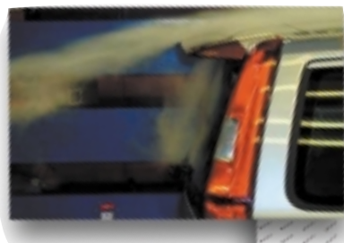
Figure 2: Dirt deposition seen via testing and CFD simulation
