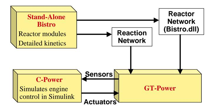
Construction of the reactor network, the reaction network, and the engine controller is done outside of the GT-Power environment, which allows each researcher to contribute specialized information).
