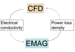
The CFD simulation leads to a stationary solution, ANSYS operates in frequency domain. The power loss density can be derived from the harmonic solution and the exchange of data between the two simulations codes is performed as soon as new results (power loss densities and conductivities) are available.
