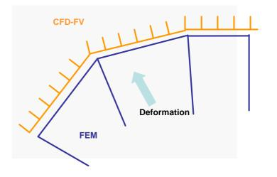
There are two ways on how to transport the latest positions of the structural surface from FEM to CFD:
