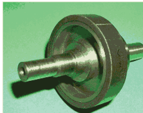
Iron cored Halbach rotor
