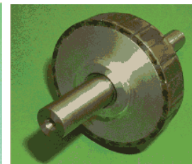
Segmented Halbach rotor
