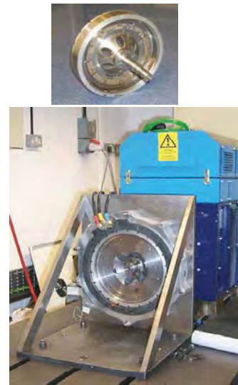
3-phase, 22-poles, 24-slots, PM brushless torque-boost machine, rated output power = 18.5kW, speed = 1700rpm, & torque = 105Nm
