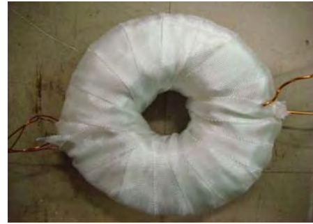
Fig. 2 Test piece to measure at high temperatures
