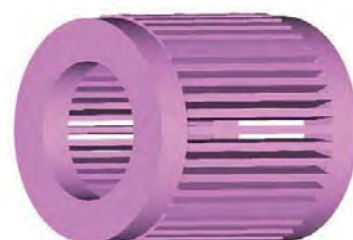
Rotor bar end rings (aluminum)
