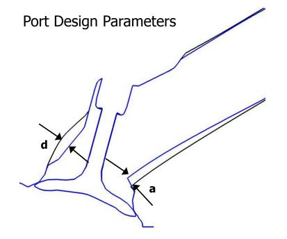
Effects of design parameters 'a' and 'd' on tumble ratio (TR) and turbulence intensity(U') at TDC, 1500rpm-2.62bar BMEP:
