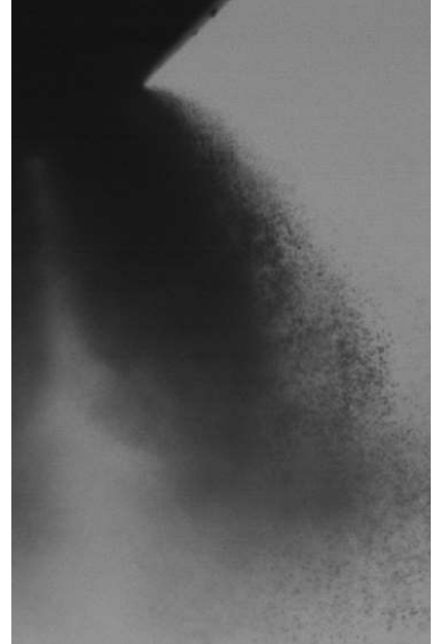
Spray with promptly phase transition (flash-boiling)
