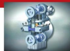
The design of Achates' opposed-piston engine in a rendered 3D model.
