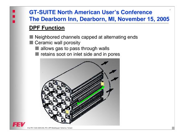
Wall flow type filters consist of a ceramic substrate, the channels which are \* capped alternatingly either at one or the \* other end. The gas has to \* pass the porous walls, and soot and other particles will stick either in the pores and/or form a cake on the walls of the inlet channels.
