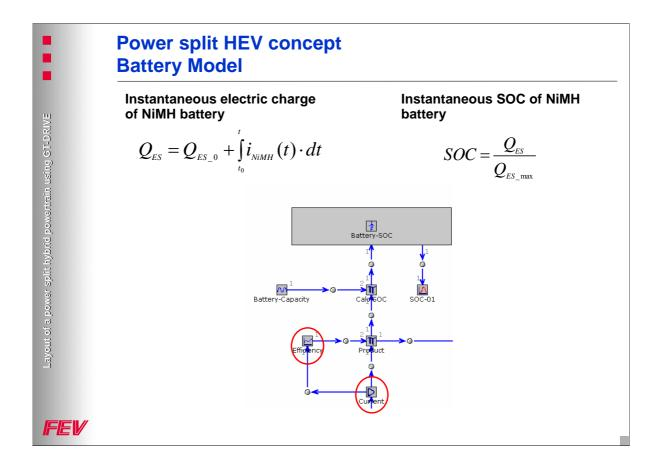
The battery model can be set up simply by integrating the battery current. The efficiency for charging and discharging is defined using a map. This simple model does not yet include a model for battery temperature and voltage. However, investigations for several vehicle concepts have shown that this simple modeling is accurate enough for the layout of a HEV vehicle.
