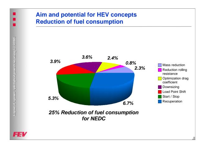
The overall potential for reducing the fuel consumption in NEDC driving cycle by using a HEV concept is about 25%. The main potential and the main aim for HEV concepts is load point shift, start / stop strategy and recuperation, which means storing the braking energy for its later use in acceleration mode.
