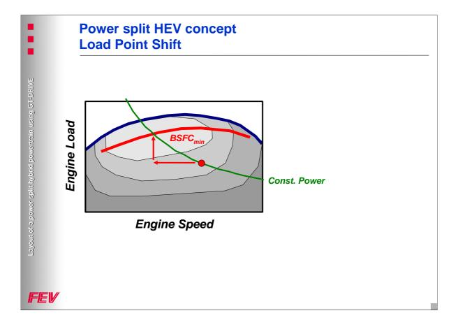
The main reason for using an electrical CVT is to enable load point shifting. For a specific vehicle speed and power demand the engine speed is decreased at constant ring speed by increasing the speed of the sun gear. Additionally the engine load is increased in order to meet the desired power. Controlled by the electrical engine at the sun gear, the ICE can be operated at optimal BSFC. The additional electric power generated at the sun gear is used by the electrical motor at the ring gear.
