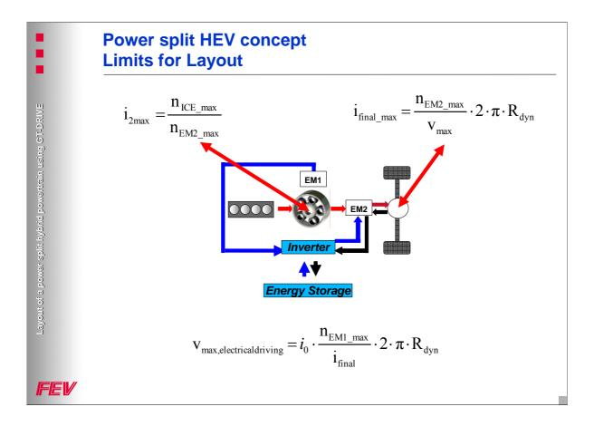
The kinematic boundary conditions of the planetary gear define some boundary conditions for the layout of final drive and planetary gear. Additionally, the maximum vehicle speeds for electrical driving is defined by planetary gear layout and maximum speeds of the electrical motors.
