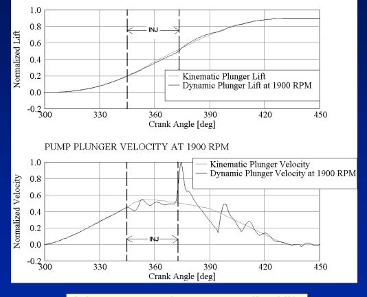
Injector pump plunger normalized lift and velocity at 1900 RPM
