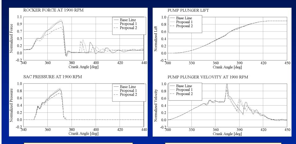
Predicted rocker force and sac pressure comparison between baseline and proposals 1 & 2 at 1900 RPM Predicted dynamic pump plunger lift and velocity comparison between baseline and proposals 1 & 2 at 1900 RPM
