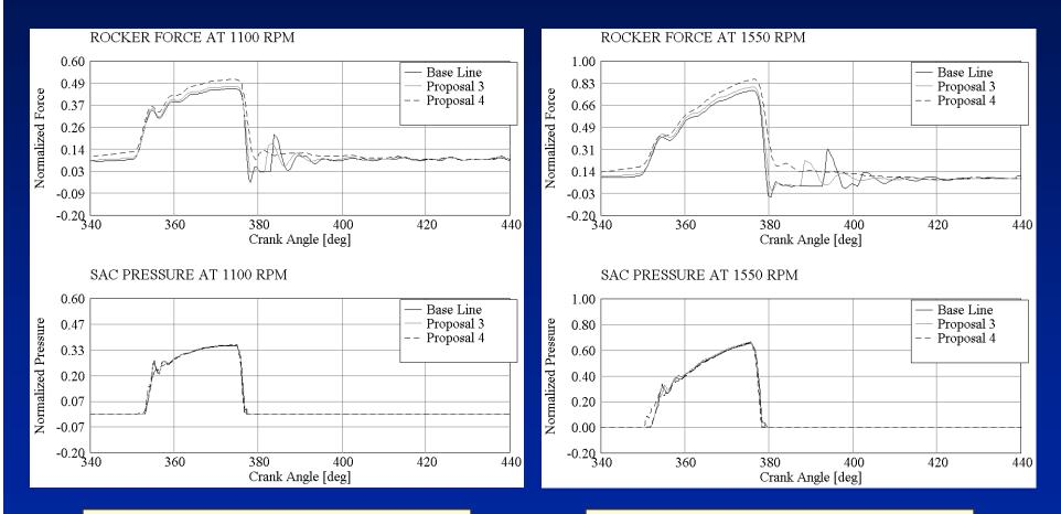
Predicted rocker force and sac pressure comparison between baseline and proposals 3 & 4 at 1100 RPM Predicted rocker force and sac pressure comparison between baseline and proposals 3 & 4 at 1550 RPM
