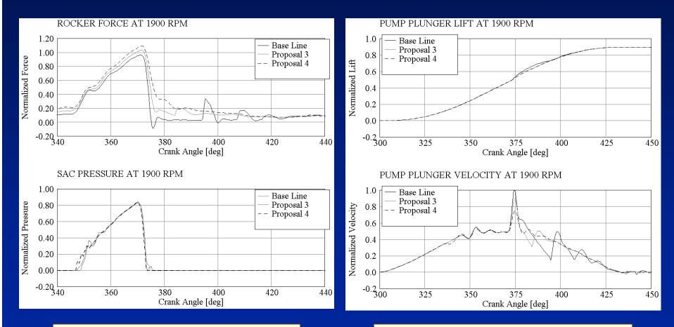
Predicted rocker force and sac pressure comparison between baseline and proposals 3 & 4 at 1900 RPM Predicted dynamic pump plunger lift and velocity comparison between baseline and proposals 3 & 4 at 1550 RPM
