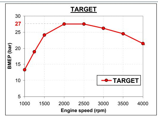
RENAULT's target: to reach 72kW/l and 220Nm/l with a smaller engine capacity (downsizing level=25%)
