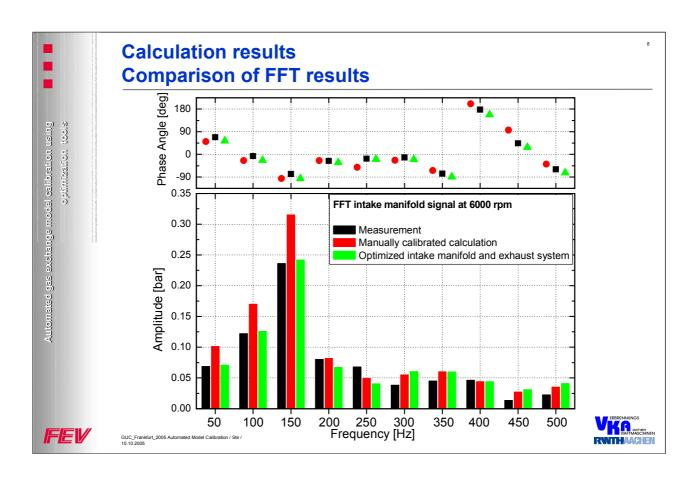
Comparing the FFT transformation results of the measurement, the manually calibrated model and the automatically optimized model, it can be seen that a significant improvement of the degree of fit can be reached for the first three frequencies. Here the fit of the automated calibration is nearly perfect. For the higher frequencies with minor influence a partly improvement was achieved.
