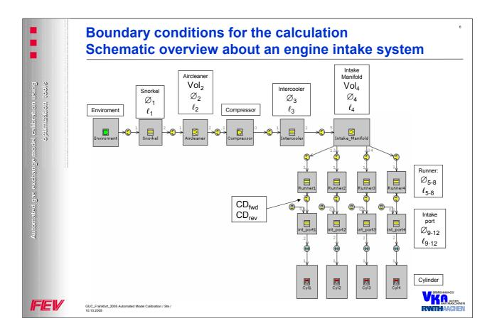
After setting the targets the input variables have to be chosen. This slide shows a schematic overview of the intake system of a turbocharged engine.
