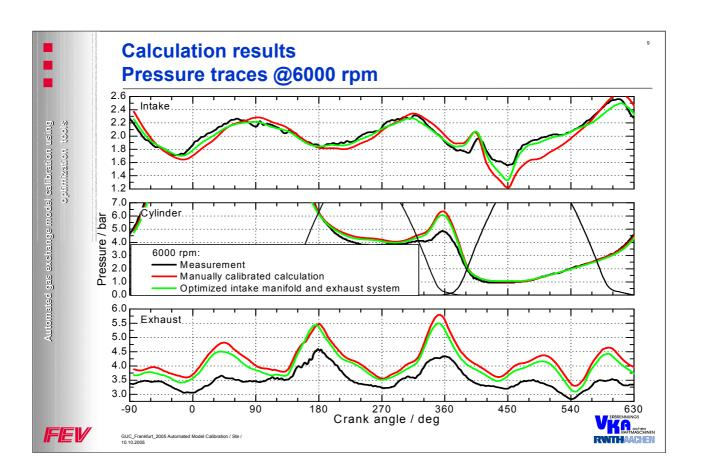
Corresponding to the FFT results, the pressure traces show a significant improvement, too. At 6000 rpm especially the suction spike during the intake phase is much closer to the measured signal compared to the manually calibrated model curve.
