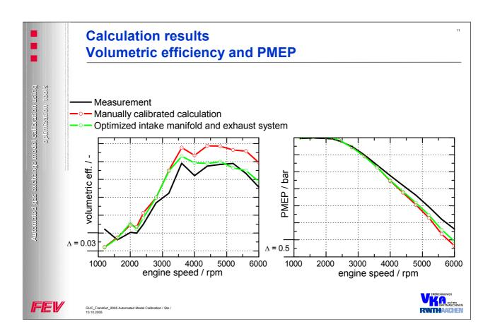
Another measure, which was not part of the optimization is the volumetric efficiency. The calculation results of the optimized model show that this measure can be improved up to 3 % in comparison to the manually calibrated model. Furthermore the pumping work could be decreased which leads to a better fit to the measurement data.
