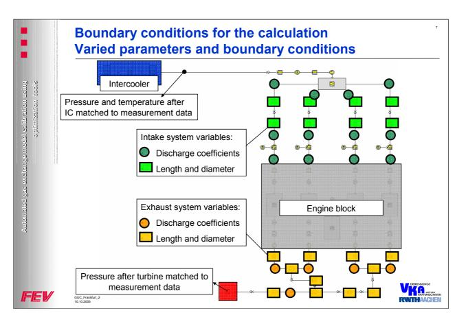
Having a look on the calculation model it can be seen that the investigation concentrates on an "inner" system. At turbocharged engines the gas dynamics before IC has got only minor influences on the gas dynamics after IC. Furthermore the turbine isolate the system on the exhaust side.
