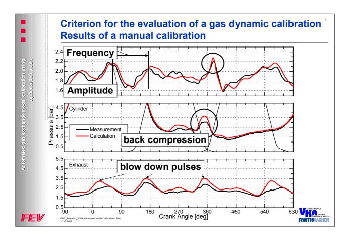
This figure shows pressure traces of the intake manifold, the cylinder and the exhaust manifold in dependency of the crank angle for a full load operation point at 3600 rpm. The black line represents measurement data while the red one is from a manually calibrated simulation model.
