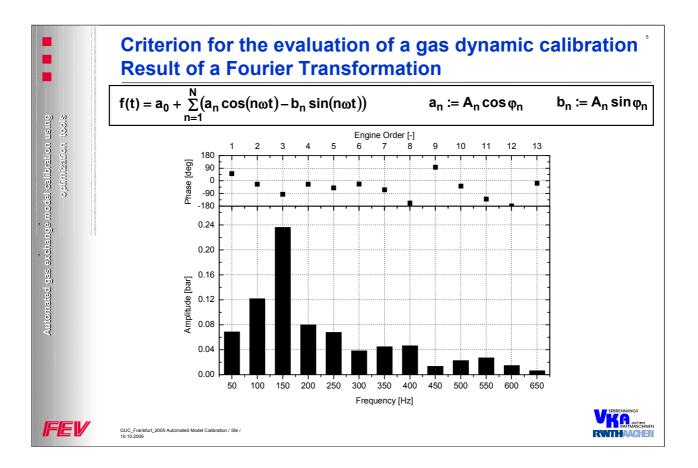
With the Fourier transformation the complex periodic pressure signal can be splitted into simple harmonic oscillations.
