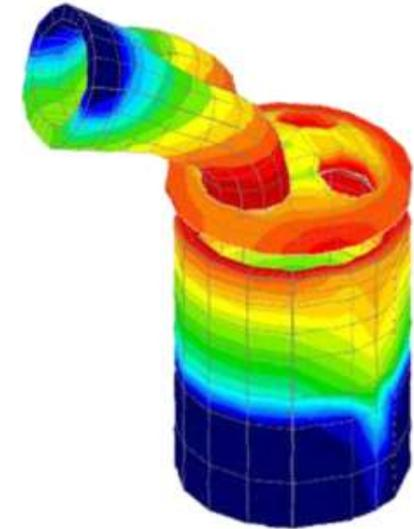
Internal cooling circuit has been built up according to most recent CAD data. GEM 3D was used to implement water jacket volumes.
