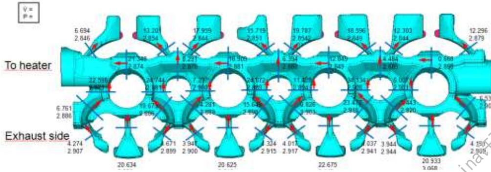
CFD results for water jacket 1D model calibration
