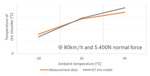
→ Difference of Rolling Resistance Factor due to different tire shoulder temperature is <5 % in the range from -20 to 40°C.
