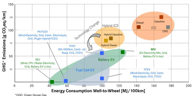
ICE = Internal combustion engine
