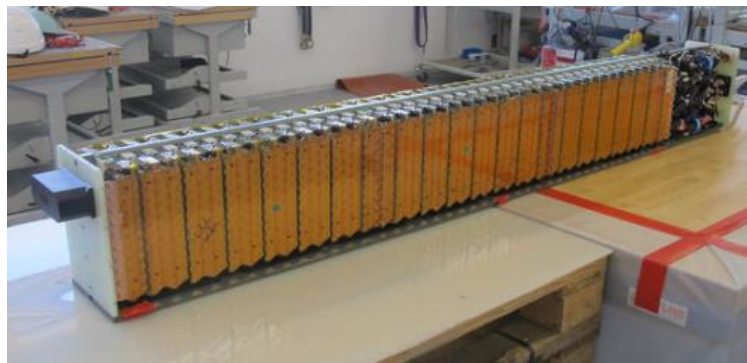
Fig 1. Picture of one of the battery packs used on the A 3 alpha flight demonstrator on a test lab bench.
