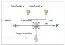
The Sub-Process Node enables users to nest processes, built with the dedicated processMODELER tool, into modeFRONTIER projects. Complex problems are converted into a breakdown of its constituent parts: modeFRONTIER workflows become modular and re-usable, natively support loop process execution and allow users to create well-organized multi-disciplinary projects.
