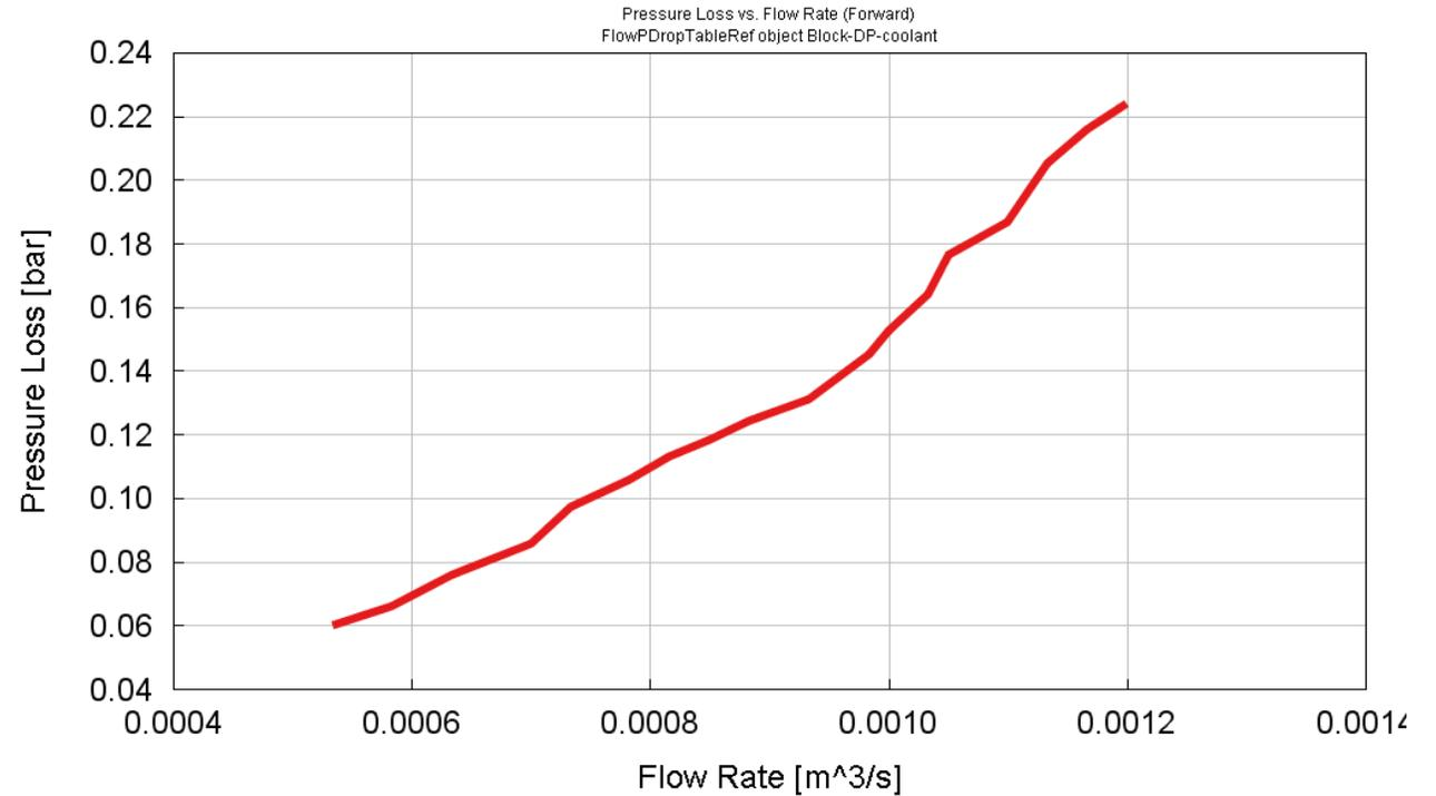
**Crankcase Restriction vs Flow is measured data in the Engine**
